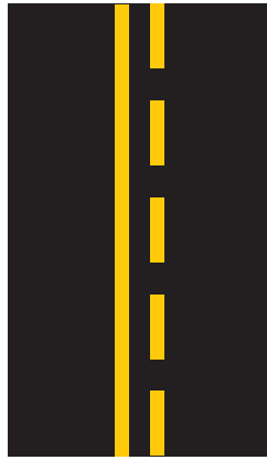
Broken line and solid line — you may pass only when it is safe and the broken line is on your side
