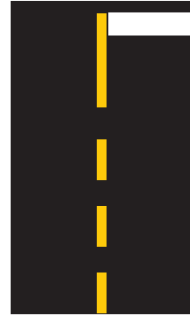
Stop line — stop before this line
