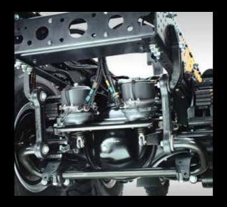
**Stability in Rear** The rear antiroll bar is also standard equipment, vital when carrying heavy loads with high centers of gravity.
