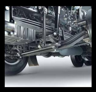
**Stability in Front** Combined with a wider wheel track, front antiroll bar increases stability, enhancing maneuverability.
