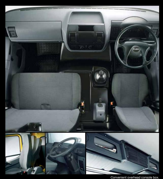
**Ergonomic, All Steel, Crash-Safe Cabin** All steel and crash safe, the FO's Extended Day Cabin is also designed for productive comfort, with fully adjustable seats, tilt-and-telescoping steering wheel, and a fold down bunk for breaks.
