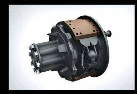
For Effective and Safe Braking Heavy duty wider and thicker brake linings of same-size on front and rear. High capacity compressor with bigger air tanks.
