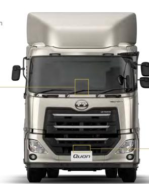
The Millimeter-wave radar functions as the main sensor when detecting the vehicle
