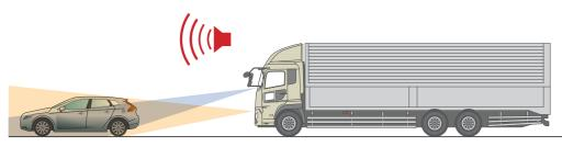
3. If the vehicle gets close enough for a collision to be possible, the system quickly applies the brakes to reduce the potential damage from a collision
