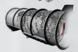
The discharge end of the rotor now includes a "corn ring" to help move crop around the cage. This promotes proper crop flow from the separation area of the rotor into the discharge.
