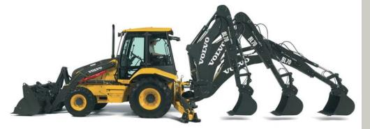
• Flow sharing load-sensing hydraulics.
