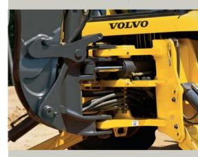
High-mounted dual swing cylinders: out of the dirt.
