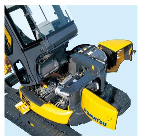
Rear bonnets for quick engine checks, simple inspections, cleaning of the radiators and easy access to the battery.
