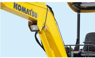
This travel lamp provides an increased visibility both in a night operation and in the travel position.
